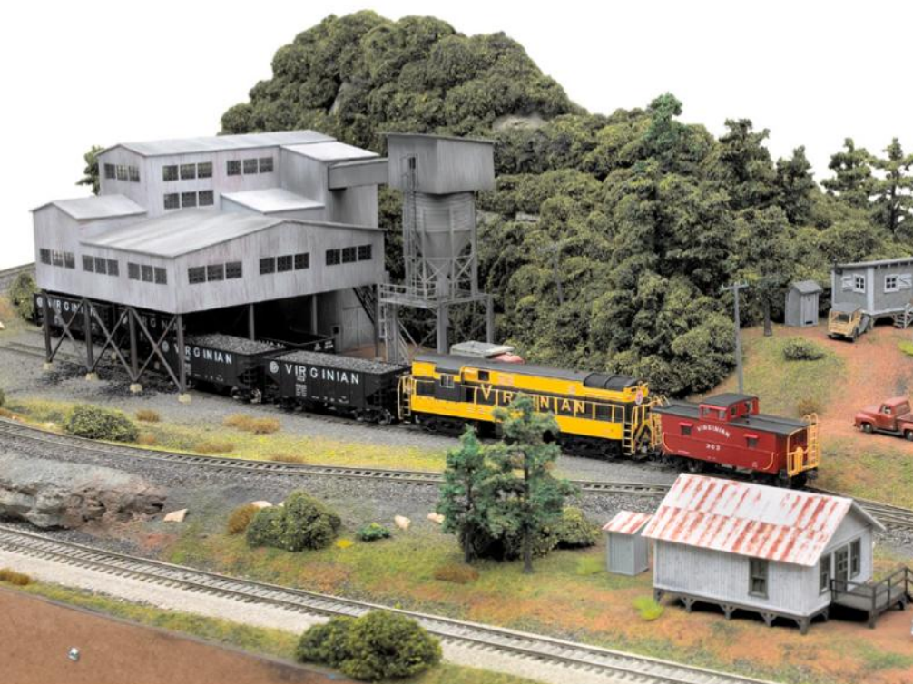
Switching a stub-ended industrial spur, like those under the coal tippie on MR's HO scale Virginian project railroad, can sometimes require a runaround move to shove the cars into the spur ahead of the locomotive. Engineers on the prototype usually prefer to avoid such maneuvers. Bill Zuback photo
