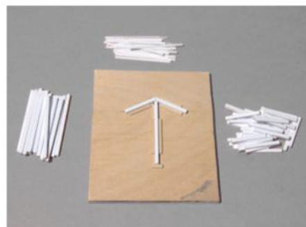
Fig. 2 Mass production. Doug built a wooden jig to assist in building the 29 supports. He cut like parts at the same time to ensure uniformity.
