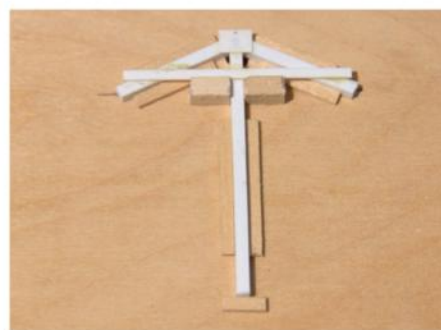
Fig. 3 Ascenders assembled. Doug trimmed the horizontal braces and top gusset plates after letting the glue dry and removing the support from the jig.
