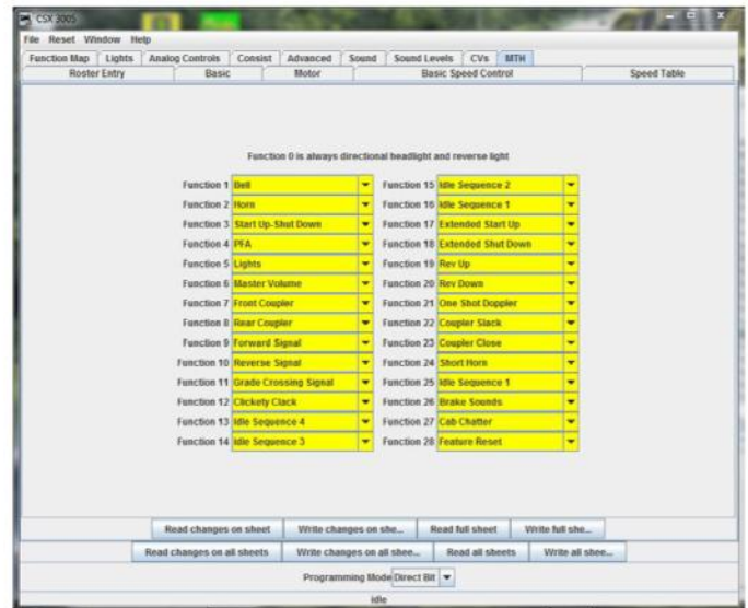
Fig. 4. Drop-down menus. The DecoderPro function mapping pane for MTH decoders presents the function buttons with a drop-down menu of effects next to each. The various function mapping panes look different to take advantage of each decoder's unique features.
