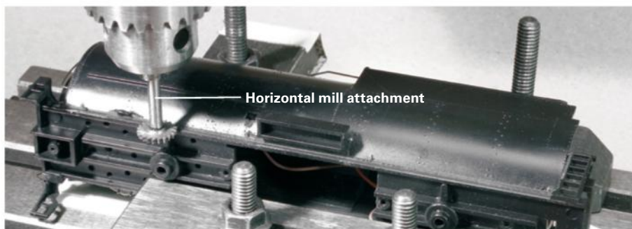
Fig. 15 A close shave. Peter removed the molded piping and rerail frog with a horizontal mill attachment in a drill press. The drill press should be run at low speed to avoid melting the plastic.
