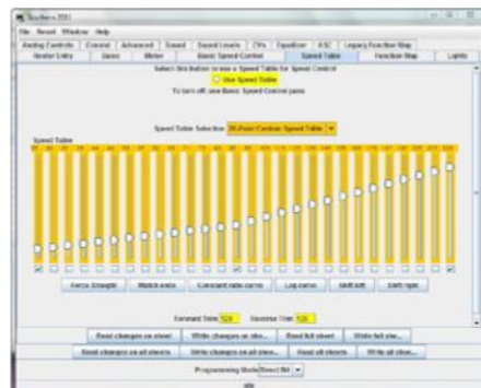
Fig. 2. Fancier footwork. Using the Speed Table pane, you can create a three-step curve by designating speeds for steps 1, 14 and 28 and straight-lining the steps between.
