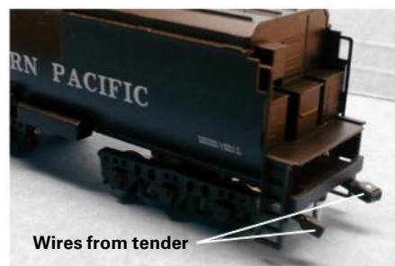
Fig. 12 Running wires. Peter cut notches in the bulkhead for the wires that run from the tender to the engine.
