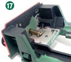
The coupling hook pokes through the bufferbeam. A spring is fitted over the shank and retained with a washer and split pin. This is a fiddly job where an extra pair of hands could be useful.
