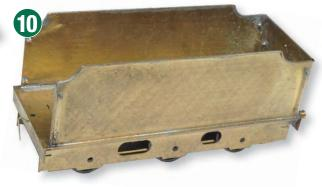
With every tender locomotive I build, I erect the two parts at the same time. This ensures mutual compatibility and ease of adjustment, if necessary, at an early stage. The tender sides and rear folded up together as one unit, perfectly. The handrails have been soldered in place before the top was attached.
