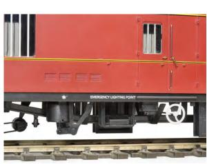
The underframe of the model. A little daylight can be seen between the trussing and chassis. The battery boxes hang a little too low, but not enough to offend the eye.
