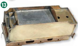
Since all my models run with a coal load, I see little point in wasting time making up the self-trimming interior. A piece of sheet lead was substituted, fixed in with low-melt solder. The lead also acts as ballast.
