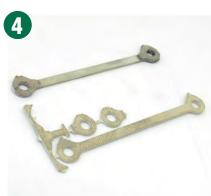
Connecting rods are etched nickel silver and require cutting from the fret with a large knife and then the bosses fitting to the ends. Solder or superglue will work for this.
