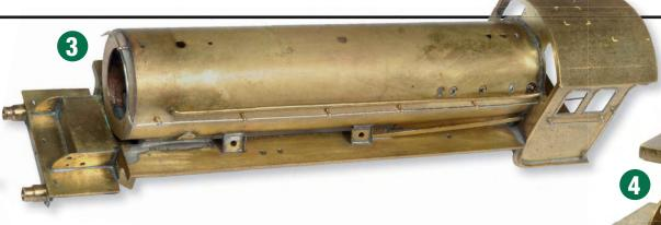
Above Cab roof on, cab window beading installed and the continuous handrail in place. It's important that stages are carefully followed to ensure that most soldering, if possible, takes place from the inside.
