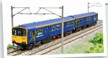
One of the two Class 150/1s is sacrificed to provide the parts to make a new centre car, a process known as cut-and-shut. A Class 150/2 could also be used, with the sliding cab door mouldings saved for the DMS and DMSL.
