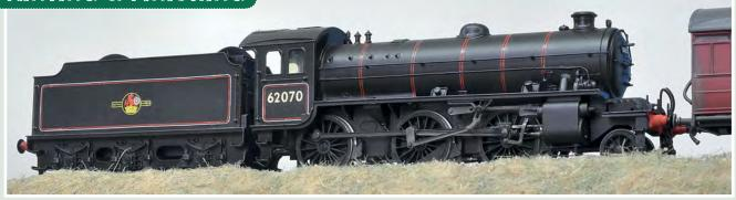
Painting was accomplished using Halfords satin black acrylic car spray, with lining by Modelmaster products and numerals/branding from the HMRS BR sheet. The front numberplate is from lan Wilson's Pacific Models range. The valance lining has yet to be applied (no curve on the transfer sheet matches the curve on the footplate, so I'll have to devise a solution). A shedplate is yet to be fitted. No. 62070 was allocated to March from new until the autumn of 1958, thence
