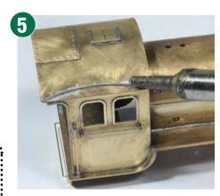
Some soldering has to be done externally, such as the cab roof rainstrips. The trick was to use as little solder as possible and flood everything with flux.
