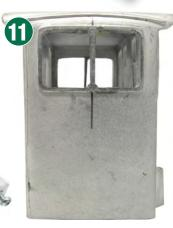
An easily missed detail is the small whitemetal pieces for the central bars in the side windows. Take time to ensure they are right in the middle and vertical in the window.
