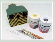
On the back I carefully marked out the stripes and painted them with acrylic paint. A plastic card template the width of a strip helped and I ran a bow pen along this to give me a sharp edge. The middle of the stripe was filled in with a brush. Acrylic paint is excellent for this work as it dries very quickly allowing rapid touch-up where mistakes have been made. Two hours and only a little bad language saw this end complete.
