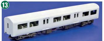
The underframe is test fitted once again, this time with the spare seating mouldings used to remove the tip-up seats fitted to the cab end of the underframe.
