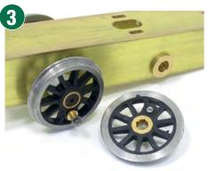
Crank pins are made up by screwing a bolt through the back of the wheel, then slipping the brass bush over this. Retain the lot with a washer and small nut. These last two are removed while fitting the connecting rods but it's worth keeping them on for the moment.
