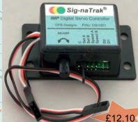
The IMP (part no: DSI1001). Drives a model control servo (with DCC or DC) for semaphore signals, or crossing gates etc.
