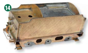
With just a few bits to go on, the basic tender work was completed very easily. Note how I've tinned the frames to allow the soldering-on of the axleboxes later.
