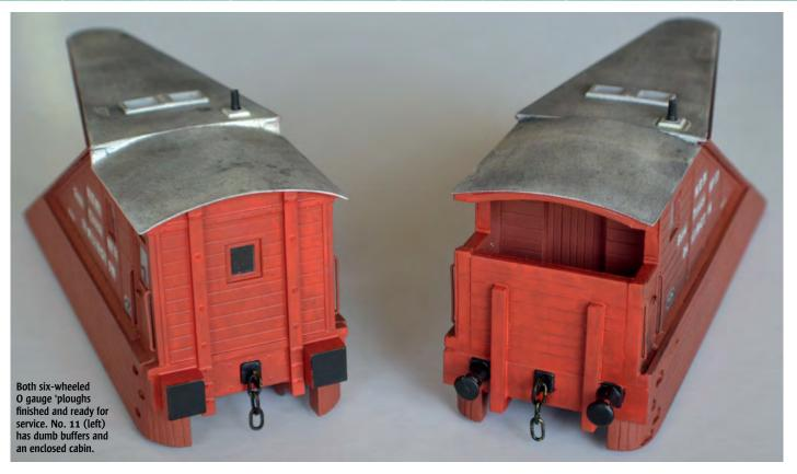
between 15 and 18 tons for four-wheeled 'ploughs. The vehicles consisted of a large ploughshare sloping upwards at about 30 degrees from the horizontal. This was bisected by a prow designed to throw the snow to either side of the line. At the rear was the cabin containing equipment and crew accommodation.
