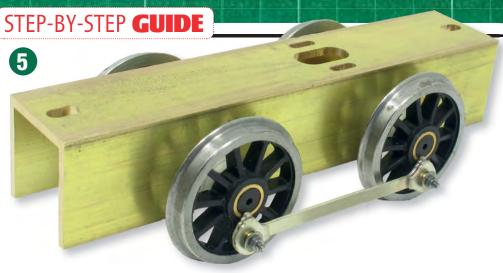
With the rods fitted, the chassis should run smoothly with no binding. If it doesn't, check the wheels rotate freely and that the rods are a slightly loose fit on the crank pins. The tolerances are generous enough that you are unlikely to encounter any problems but if you do, check your assembly before enlarging any holes.
