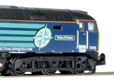
models have been upgraded with a sixpin DCC decoder socket. As before, the '57' has directional LED head and tail lights, all-wheel pick-up and drive and Rapido type couplers in NEM pockets.
