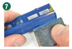
The roof hatch detail is carefully rubbed away with grade 1200 'wet and dry' paper to leave as much of the roof rib moulding as possible. The gaps in the ribs are filled with 10thou square styrene strip.
