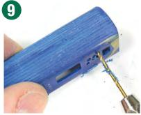
A 2mm drill and scalpel blade is used to open out the window. A moulded glazing unit is used to check the required size when finishing the opening.
