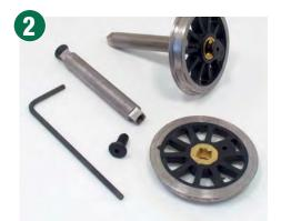
Test fit the wheels to the axles. The supplied Allen key is used to turn the retaining screws in the middle. Put this somewhere safe as it's easy to lose. Wheels should be 'quartered'; in other words the crank pins on an axle are set at 90 degrees (one quarter turn) from each other.
