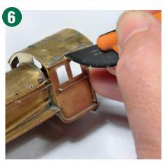
Even then, external solder has to be removed - most easily to begin with using the tip of a craft knife. It's a pity spectacle beading was not included as part of the kit.
