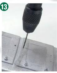
There are lots of holes to be drilled for handrails. All are marked with little dimples in the casting and should be opened out with a 0.7mm drill. This can bind in the metal but a little spit on the bit will lubricate it.
