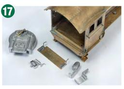
The cab interior components were made up and are ready to be fixed in place. The lifting fallplate is a very good idea.
