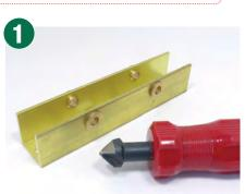
The instructions state "Remove any machine burrs from the chassis". This just means making sure the axle holes are clear of any residue. A small round file will be fine for this but if you have a countersink drill bit. it's even easier to rotate this in each hole. Check the bearings fit and run a little superglue around the edge to hold them in place.
