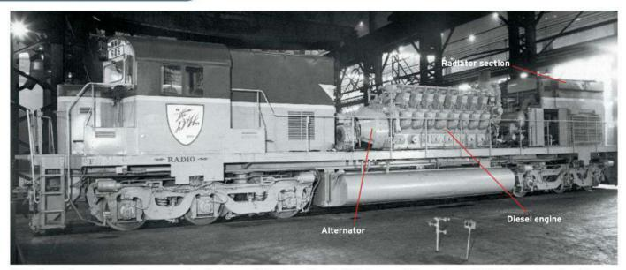
With its engine-room hood removed, a Delaware & Hudson Alco C-628 shows off its series 251C V-16 diesel engine. The diesel drives the alternator to produce electricity for the unit's axle-mounted traction motors. Jim Shaughnessy photo
