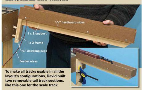
**BECAUSE WE BUILT THE LAYOUT** to be used in any of three configurations (See the January 2010 MR), in some setups, we have one or two tracks that need to be extended to be useful. I made two removable tail tracks, one for the scale track and one for the runaround track by the Blatz warehouse. These temporary tail tracks plug into the layout when needed, are held in place with a clamp, and have a set of feeder wires that plug into the track bus.
