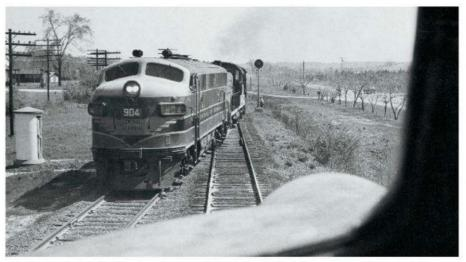
Photographer J. Parker Lamb was aboard Central of Georgia southbound time freight No. 34 when it met No. 29 at Smith's, Ala., in March 1955. The automatic block signal provided safety but didn't convey authority for train movements.
