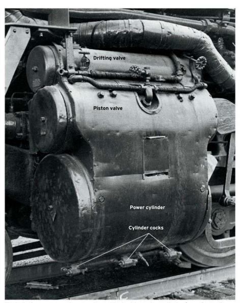
Typical of most steam locomotives, this double-acting cylinder (on a Santa Fe 2-10-4) both produces power and releases exhaust steam on each stroke forward or backward. The engine's two cylinders exhaust a total of four times for each revolution of the drivers. Trains photo by Harold A. Edmonsen
