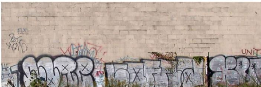
Fig. 2 Squared image. In this view Lance squared the wall by correcting for the barrel effect and perspective distortion. Copying and pasting plain images of adjacent blocks covers the undesirable pipe, shrubs, and weeds.
