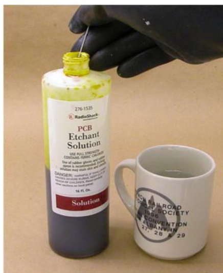
Fig. 11 Etched details. The items shown above include .055" steel music wire that Lance painted, chipped, and etched; 1/32" aluminum rod with light etching; and .025" music wire etched and allowed to rust naturally. Eye protection and proper safety precautions are necessary to safely handle the hazardous ferric chloride etchant solution he uses to speed up the natural weathering process.
