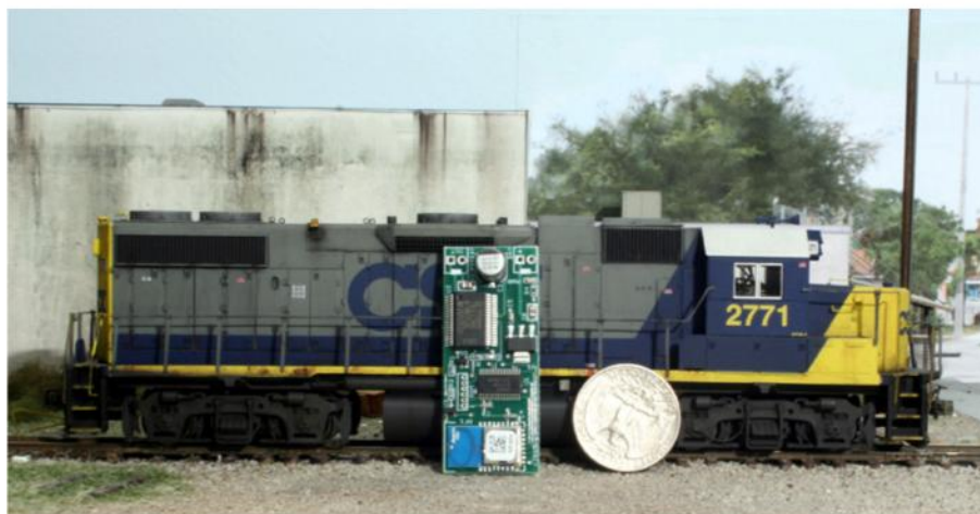
The CONVRTR from CVP is a miniature radio receiver along with a DCC booster packed into a tiny 0.8" x 2.0" circuit board. The device allows battery power controlled by the same DCC wireless throttles that run a rail-powered system.
