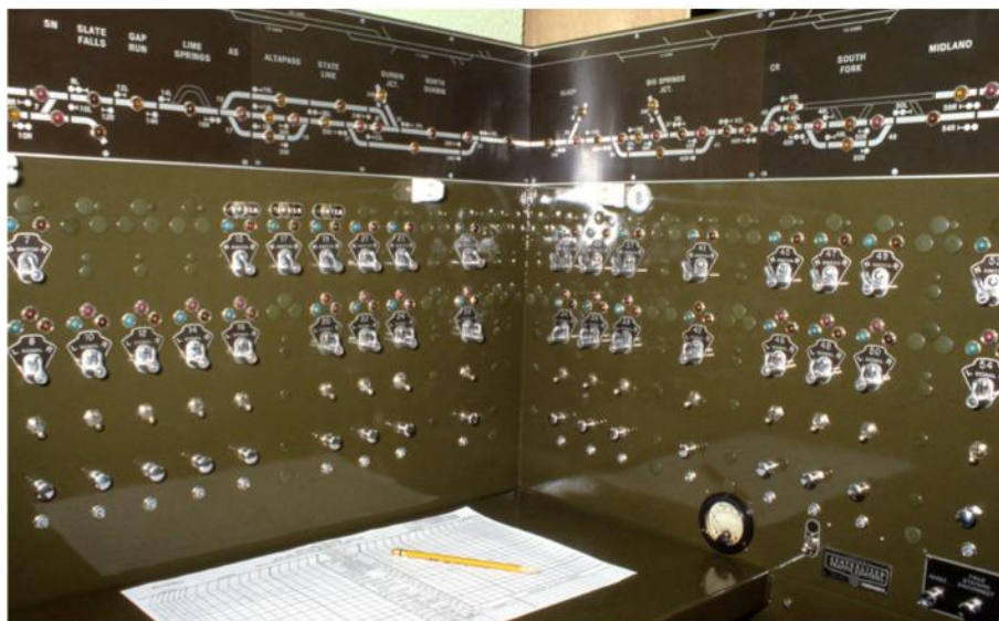
The AM was dispatched using an authentic Union Switch & Signal CTC machine, "kitbashed" from salvaged parts by Rod Loder. It was never fully operational but still provided a realistic job for the dispatcher.
