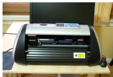
Lance's Black Cat electronic die cutting machine allows him to quickly cut highly accurate paint masks and structure veneers out of .020" styrene.
