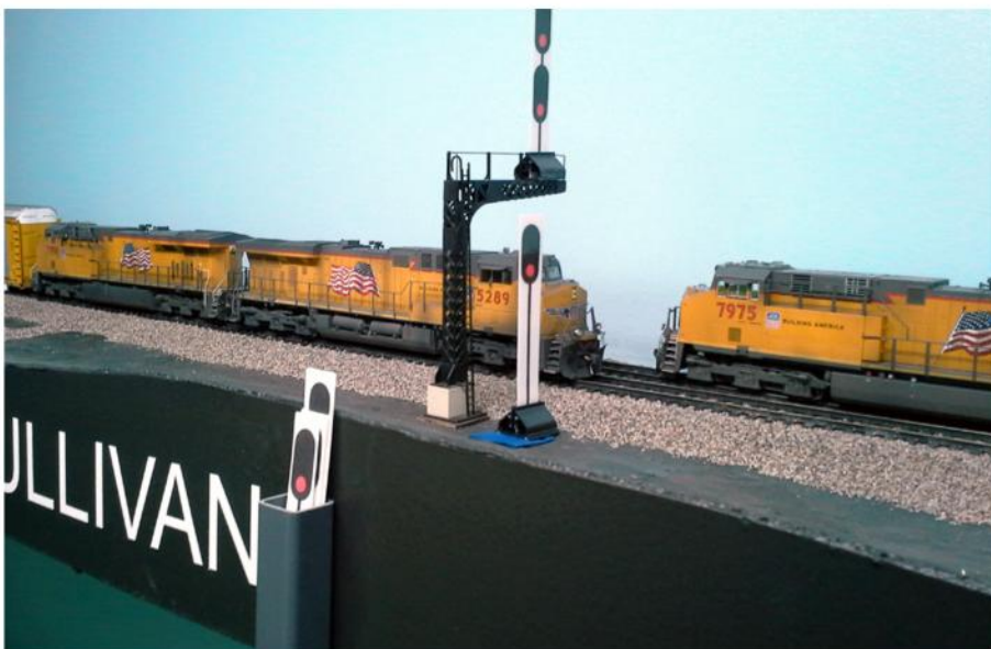
Fig. 5 A meet in progress. Union Pacific 5289 meets UP 7995 at West Sullivan, Kan. Bruce's friend Phil Buck installed a signal bridge for the siding. The signal on the ground is for the main line. The signals are placed at the fouling point of the two tracks. Note the spare signals in the holder, attached to the fascia.
