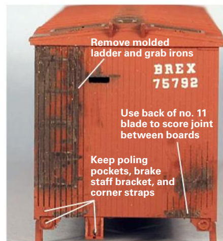
Fig. 4 A close shave. Mont removed many of the molded end details using a no. 17 chisel blade and a hobby knife. He left some of the cast details near the bottom of the car.
