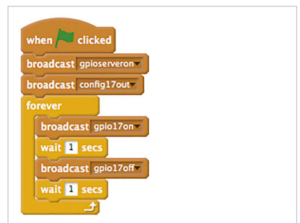
A simple script to make an LED on pin 17 blink on and off
