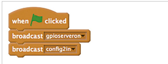
A Scratch script that can be used to initialise an input component
