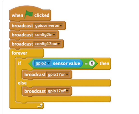
A Scratch script to light an LED whenever a button is pushed
