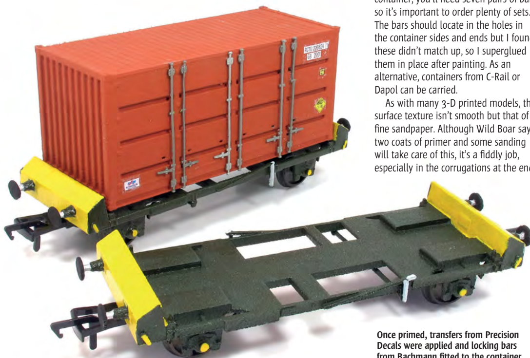
The kit is printed in polyamide, described by the manufacturer, i.materialise, as a white, very fine, granular powder that is strong, somewhat flexible and can take small impacts and resist some pressure while being bent. The surface has a sandy, granular look, and is slightly porous.
