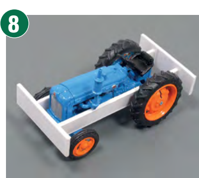
A much simpler set of buffing gear here. 5mm deep strips of 1mm thick plastic are notched to be level when fitted to the top of the axles. 24mm long buffer beams from the same material are just wide enough to match the width of the buffers on a standard gauge wagon.
