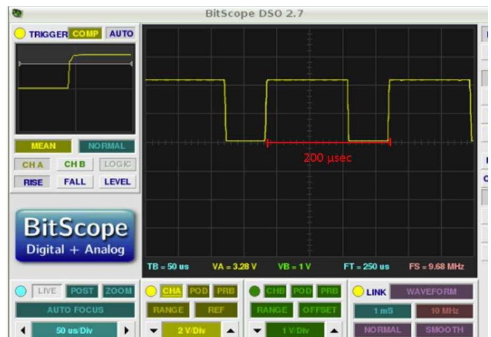
Fig. 8: Output of the clock generator circuit
