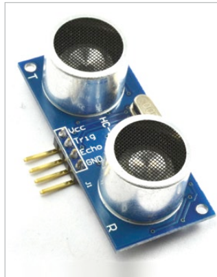
Left The HC-SR04 Ultrasonic Rangefinder. Cheap-as-chips sonar
