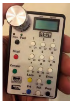
ABOVE: The MERG DCC system offers a more cost-effective way to enter the world of DCC, compared to off the shelf system. Its main advantage is its compatibility with the CANBUS system.
