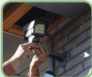
Christoph's smart surveillance project places a Raspberry Pi and Camera Module inside a fake CCTV camera housing
