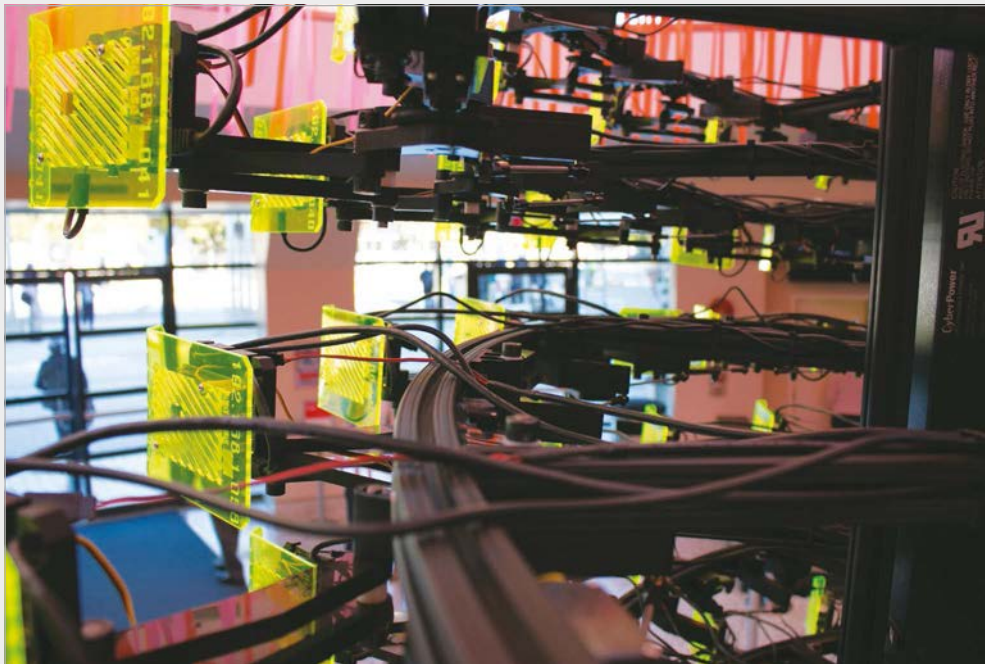
Above Each panel moves out in proportion to its Pi's workload
