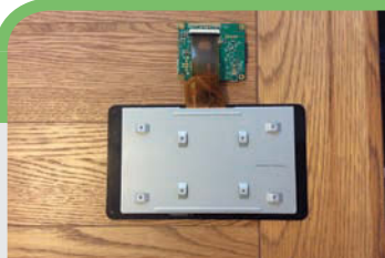
Connect the screen's wide ribbon cable to the port on the rear of the video board.
