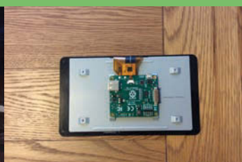
Lie the board on the back of the display and connect the small ribbon to the J4 port.
