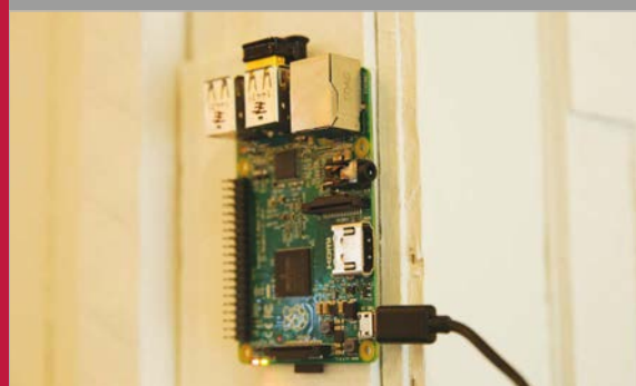
The Estimote beacon transmits a steady ping that can be picked up by the Raspberry Pi
