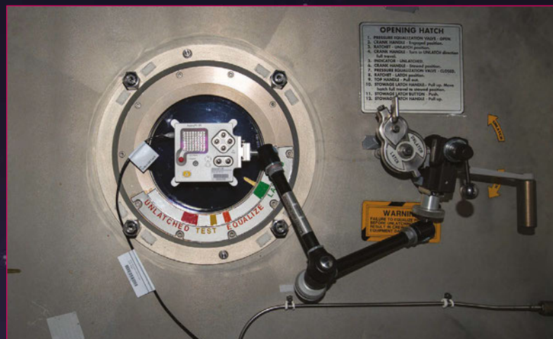
Credit: ESA In order to get a good image of Earth, Tim Peake stuck the Astro Pi IR device onto the hatch window of the ISS
