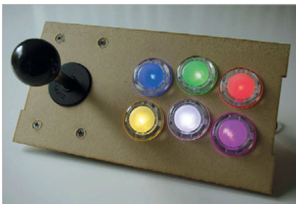
Above Whilst not in this guide for simplicity, putting NeoPixels inside the buttons adds some pizzazz to the RaspCade
