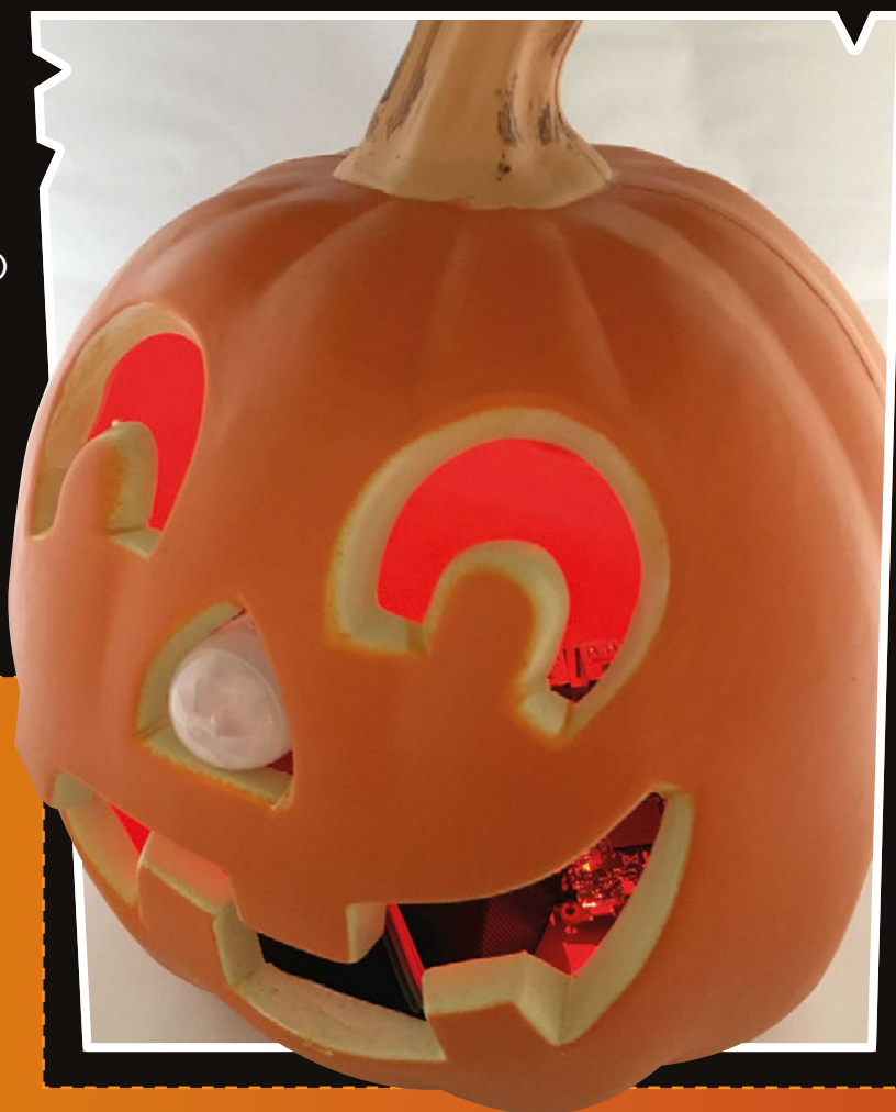
Above With a portable charger it's possible to embed the Raspberry Pi inside a pumpkin. Just make sure the PIR sensor can view the outside. (image: Daryl Mitchel, Flickr)
