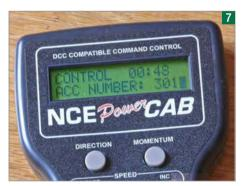
Press 'Select Acc' and key in the desired number – in this case '301'. Press ENTER. Press '1' to select 'N(0N)' and toggle back and forth a few times to set the address.
