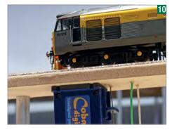
Run a train across the point. If it shorts when it hits the frog, swap the two wires to the power/accessory bus over at the terminals under the motor.
