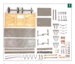
Components of the kit laid out. Parts include cast resin and laser-cut steel for W-irons, V-hangers and brake levers and cast phosphor-bronze for the axleboxes.
