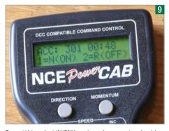
Press '1' to select 'N(ON)' again and your motor should burst into life. Press it again to change back, and check for possible obstructions.
