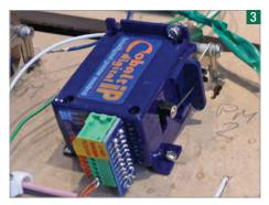
This motor is fitted with a 90deg adaptor to reduce its depth below the board. Test fit to ensure the mechanism can move freely, then fix permanently with screws.
