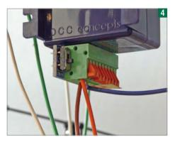
Every Cobalt motor has clearly marked push-fit terminals. I only need three wires - two to the power bus, one to the point frog (blue), switching polarity as required.
