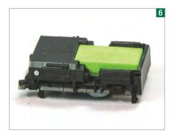
Test-fit until you're happy. The speaker enclosure shouldn't sit lower than the fuel tank. If you haven't enough room, remove more of the chassis that sits above it.
