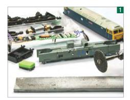
The fuel tank provides the perfect depth for the speaker, but grinding the chassis to accommodate it is a messy job. Separating the parts prevents the spread of metal dust.
