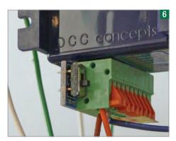
Move the switch on the motor to 'SET' and program the motor with a unique address. I'm using an NCE PowerCab, but most DCC systems have a similar process.
