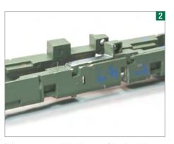
Using a tungsten-carbide disc, part of the chassis is removed. The half nearest the camera has been done. Neaten with a hand file when finished.
