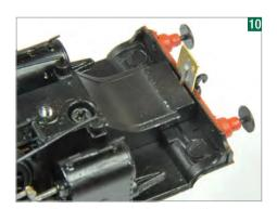
My modified model was to be fitted with AWS equipment, so a magnet protection 'bang plate' was made from brass, soldered to a brass pin and fixed with superglue.
