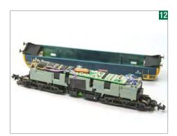
Tidy up loose wires with electrical tape and test motion, sound and lights. Paint the green speaker enclosure matt black to disguise it. Reassemble and enjoy.
