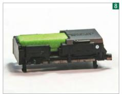
Fix the speaker into place with superglue. Ensure contact is made between the plastic of the fuel tank and the enclosure, avoiding metal parts.
