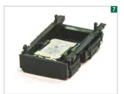
Before permanently gluing into place, take the speaker out and bend the electrical tags down so they don't sit proud of the speaker base.
