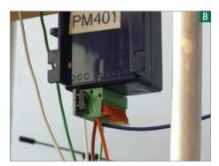
Slide the switch back to 'RUN' and the address should be set to your required address. Ensure all your connections are securely fixed.
