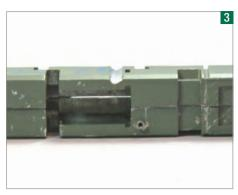
A shallow channel is made down one side of the chassis block to run the wires from the Zimo MX649N decoder to the speaker.
