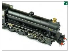
The AWS conduit on the offside footplate valance was fashioned from 15Amp fuse wire, fixed with superglue. The locomotive body remains attached to the chassis.
