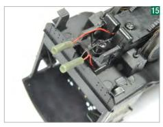
To obviate any chance of the soldered joints touching, I sleeved each one with small-bore rubber tubing. From the side, these look like tender-locomotive feeds.
