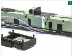
Insulate the chassis where the speaker fits to avoid shorting. This is the most common cause of sound decoder failures.
