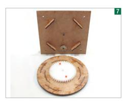
Under the disk, a large white gear is fixed with superglue. Orange plastic pins ensure it lines up with the central hole. A clear plastic gear fits to the motor without glue.
