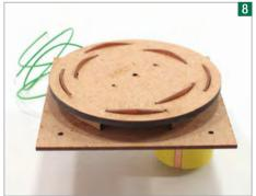
The mechanism can now be tested. The motor uses 16V AC - using DC will make it click, but not rotate and could cause damage.
