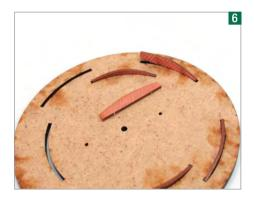
A circular plate with raised cams elevates the moles. The cams are released from their card supports and hand bent to shape.
