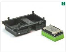
Carefully file out the opening lengthways in the fuel tank for the Limo 6mm speaker. A snug fit is a good idea as it'll hold its position better when the glue dries.
