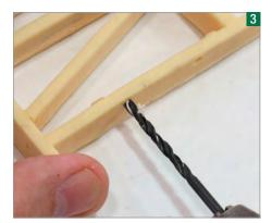
Dimples on the sides indicate where the 3mm diameter holes are to be drilled to bolt the W-irons in place. A minidrill makes short work of this.
